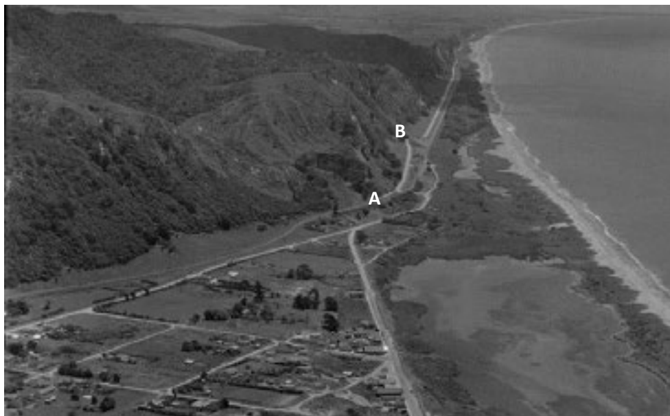
Figure 8.6: View of Matatā in 1953. Awatarariki Stream (A). Note how the former alignment of SH2 goes up and around a debris fan (B). (reproduced with permission of Alexander Turnbull Library).
