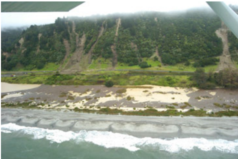
Figure 8.3: View of debris avalanche landslides on the Matatā Escarpment as a result of the rain that generated the 18 May 2005 debris flow event
