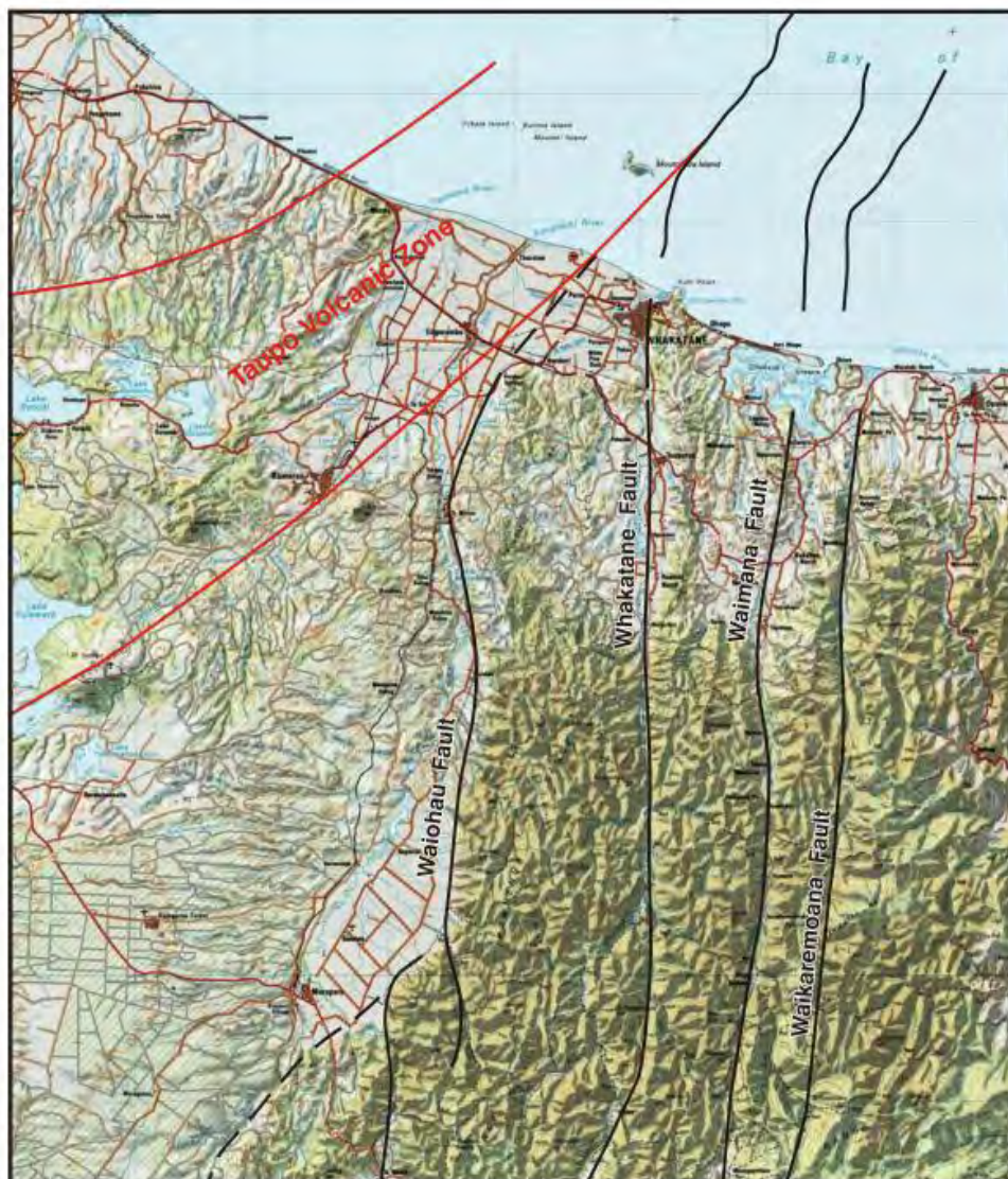
Figure 6.12: Geological structure of the eastern Bay of Plenty. Whakatane and Ohope lie at the junction of the Taupo Volcanic Zone and the North Island Shear Belt 3 (Source: Beetham et al (2000))
