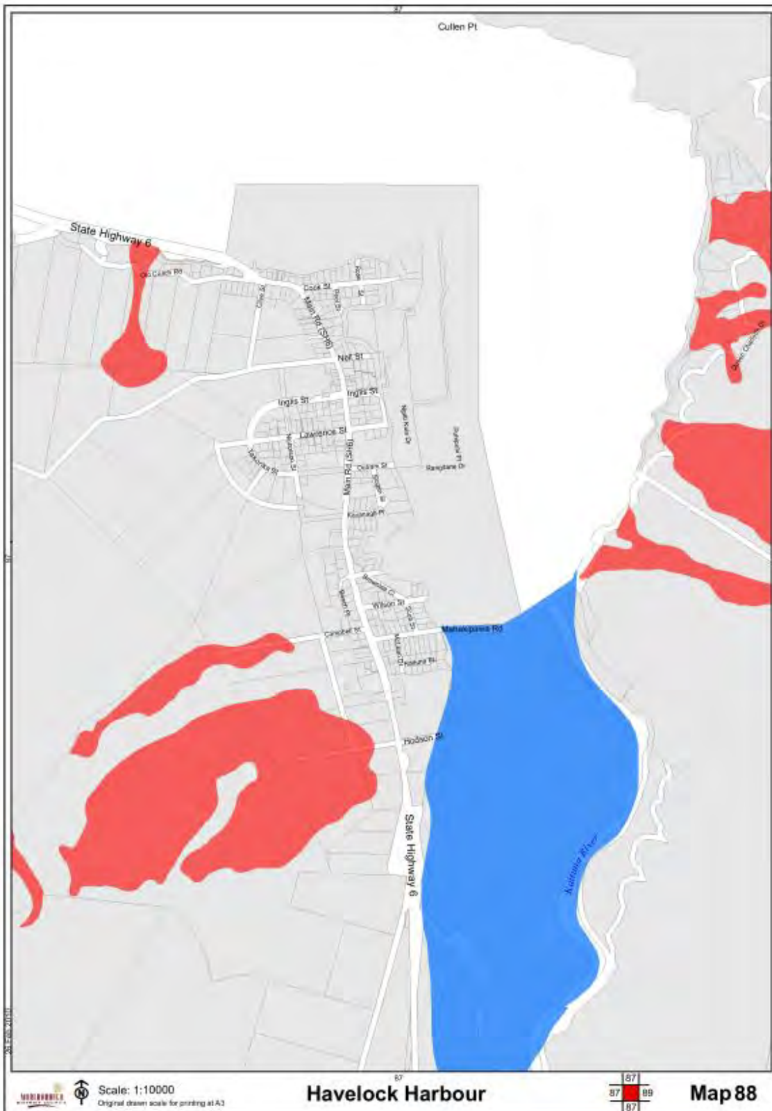
Figure 17.1: Example of a planning map showing natural hazards at property level. Areas in red are subject to land instability (Source: Marlborough Sounds Resource Management Plan).
