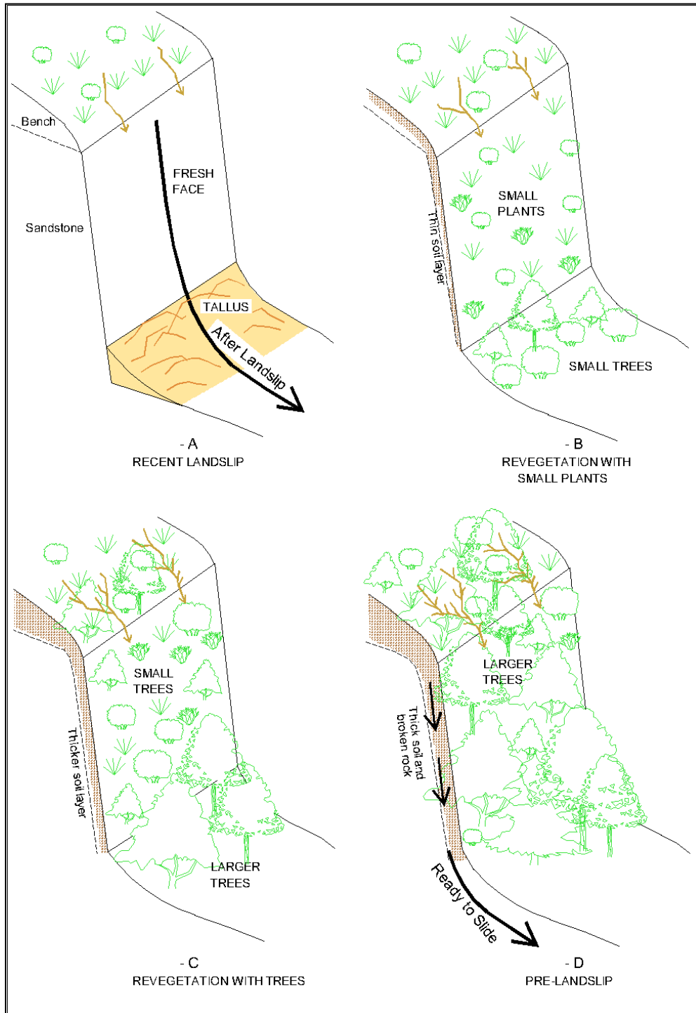
Figure 9.14: Illustration from T&T (2005) showing the natural cycle of vegetation establishment, growth and landslide on steep sections of the escarpment.
