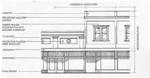
Figure 1: Typical components of late 19th and early 20th century building frontages
