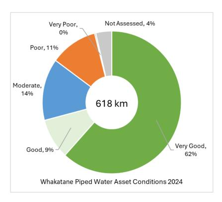
Figure 2 – Drinking water piped assets condition ratings.
