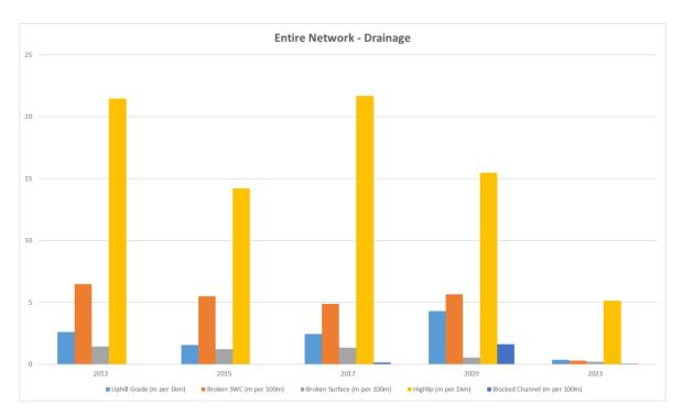
Figure 15 – Transportation Network - Drainage
