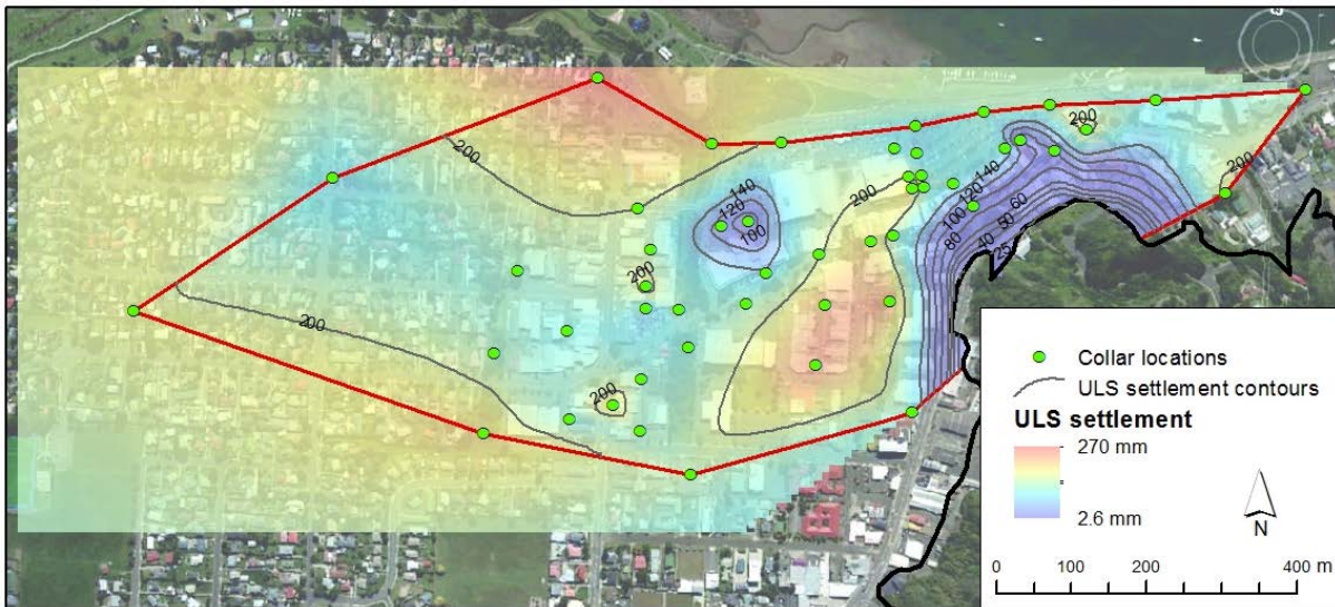
Figure 4 A map grid approximating settlement in an ULS earthquake (0.40 g, 1/500 yr event with Z=0.30 ), contoured within the zones of relative reliability (red polygon) with 25mm, 40 mm, 50 mm, 60 mm, 80 mm, 100 mm, 150 mm and 200 mm contours. CPTs that provide the primary data are displayed as green points. Comments on reliability in the caption for Figure 3 also apply here.
