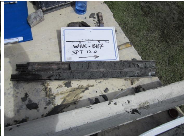
Figure 9 SPT record: WKT BH7 SPT 12m.
