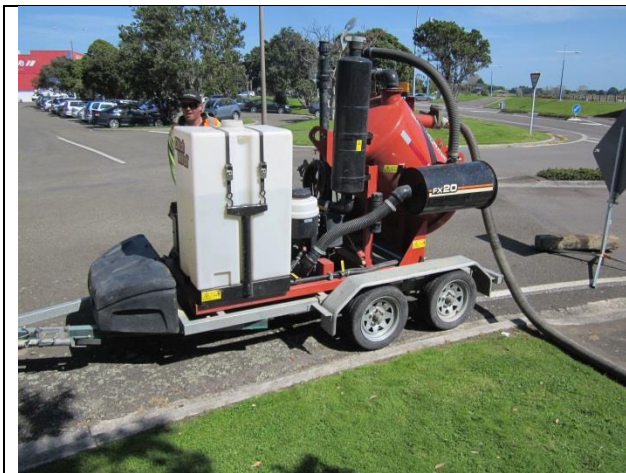
Figure 21. GEOTECH Vacuum trailer
