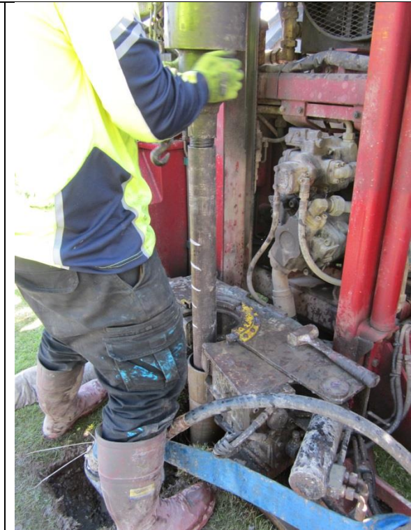
Figure 7. SPT setting up and marking 75mm intervals
