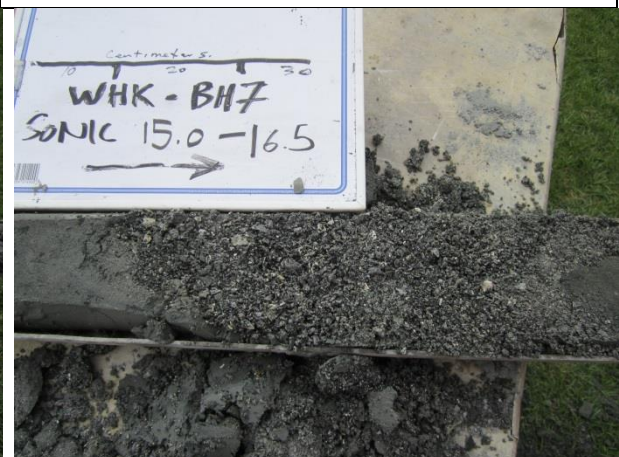
Figure 11. Close-up photo: WKT BH7 splits 15.8m shell beds
