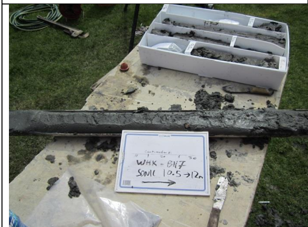
Figure 10. In situ split tube core: WKT BH7 SPT 12m.
