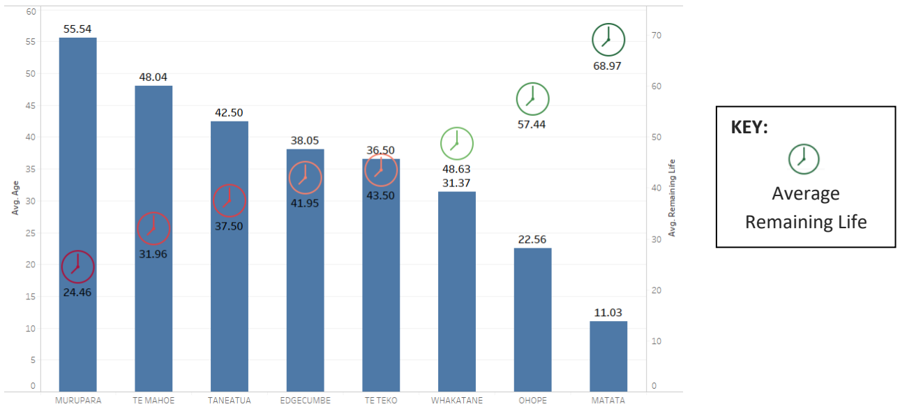
Figure 2: Manhole Average Pipe Age and Remain Life of Each Scheme*
