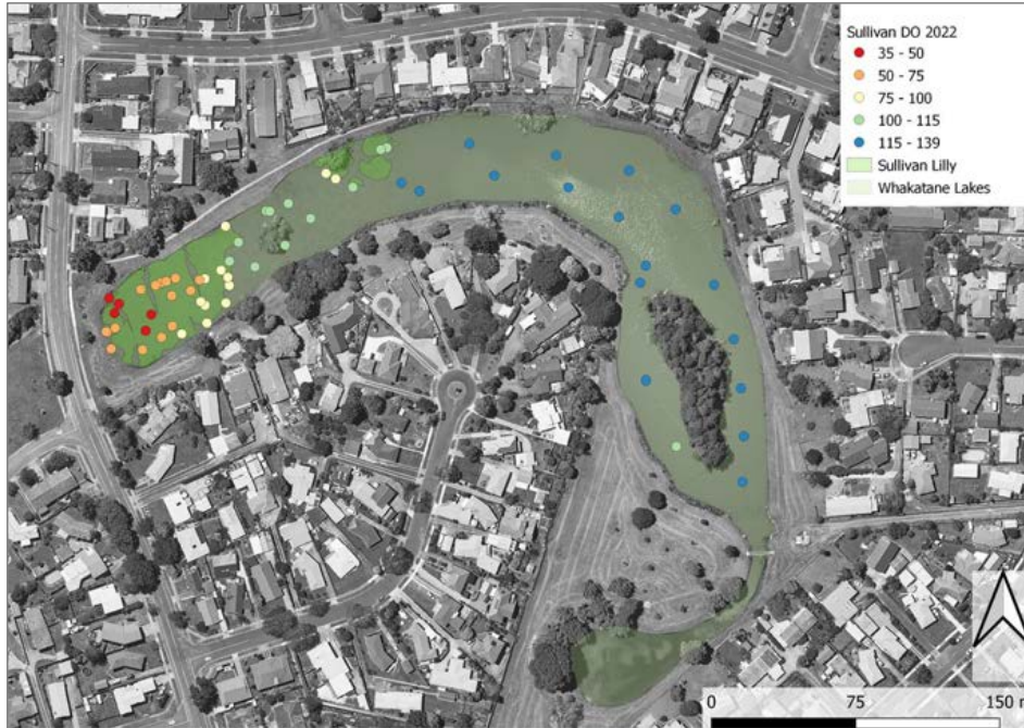
Figure 3.12: Spatial variation of dissolved oxygen in Sullivan Lake during early morning on 5 April 2022. Note super-saturation in the main body of the lagoon and low DO at the western end.
