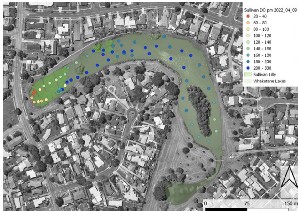
Figure 3.13: Spatial variation of dissolved oxygen in Sullivan Lake during late afternoon on 9 April 2022. Note super-saturation in the main body of the lagoon and persistent low DO at the western end.
