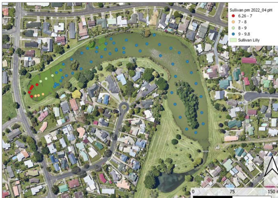
Figure 3.15: Spatial variation of pH in Sullivan Lake during late afternoon on 9 April 2022. pH is very high in the main body of the lagoon (consistent with photosynthesis) and low at the western end (consistent with respiration/decomposition).
