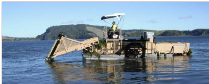
Figure 4.1: A lake macrophyte harvester in operation on Lake Rotoehu (source: www.lakeweed.co.nz ).
