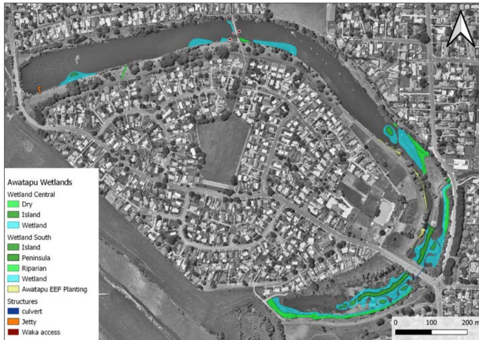
Figure 4.1: Potential layout for a treatment wetland and riparian wetlands in Awatapu Lagoon to improve water quality and provide biodiversity values.
