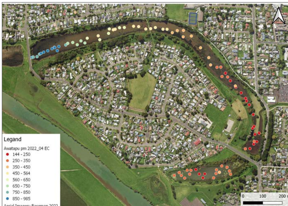
Figure 3.18: Spatial variation of electrical conductivity (uS/cm) in Awatapu Lagoon during late afternoon on 11 April 2022. EC is higher in the western lagoon due to the influence of brackish water from the Whakatāne River.
