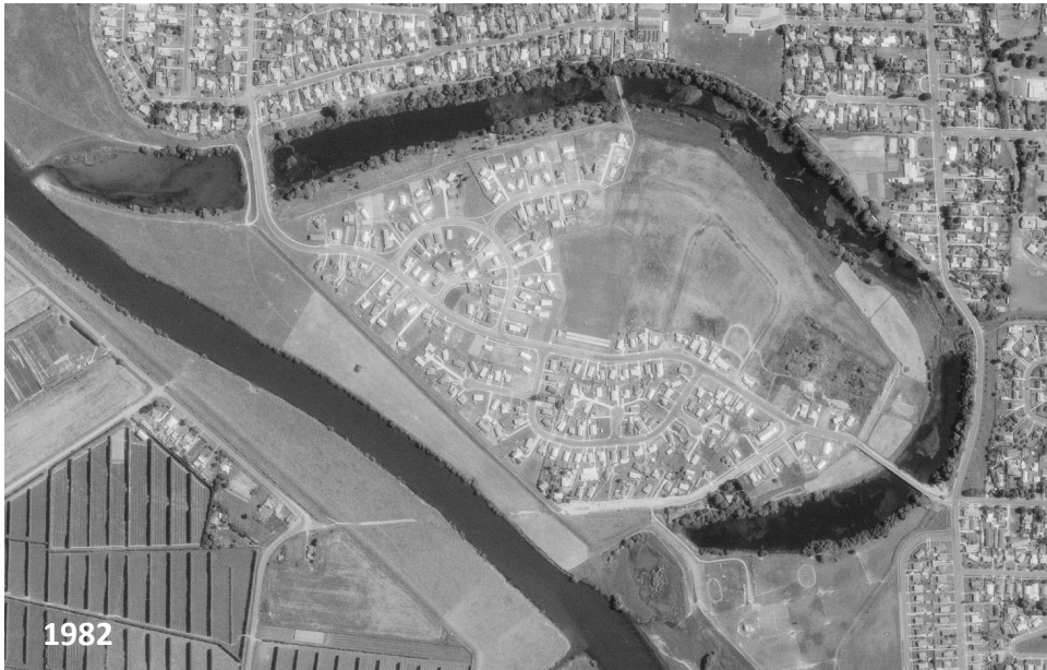
Figure 1.3: Aerial photos of Awatapu Lagoon in December 1982 showing the development of a large delta at the entrance of the Wainui Te Whara Stream (Source: Retrolens).
