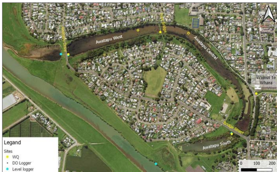
Figure 2.1: Location of water level and water quality monitoring sites in Awatapu Lagoon (aerial image: Open Commons, LINZ 2022).
