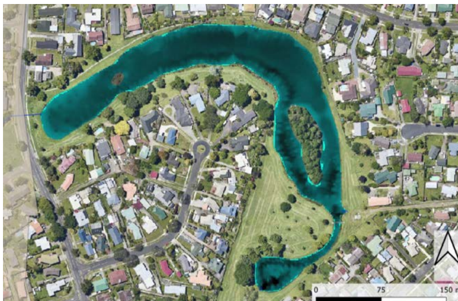
Figure 3.1: Bathymetry of Sullivan Lake. The darker areas indicate deeper water, with the maximum depth was 2.2m in the southern section and an average depth of 0.84m.
