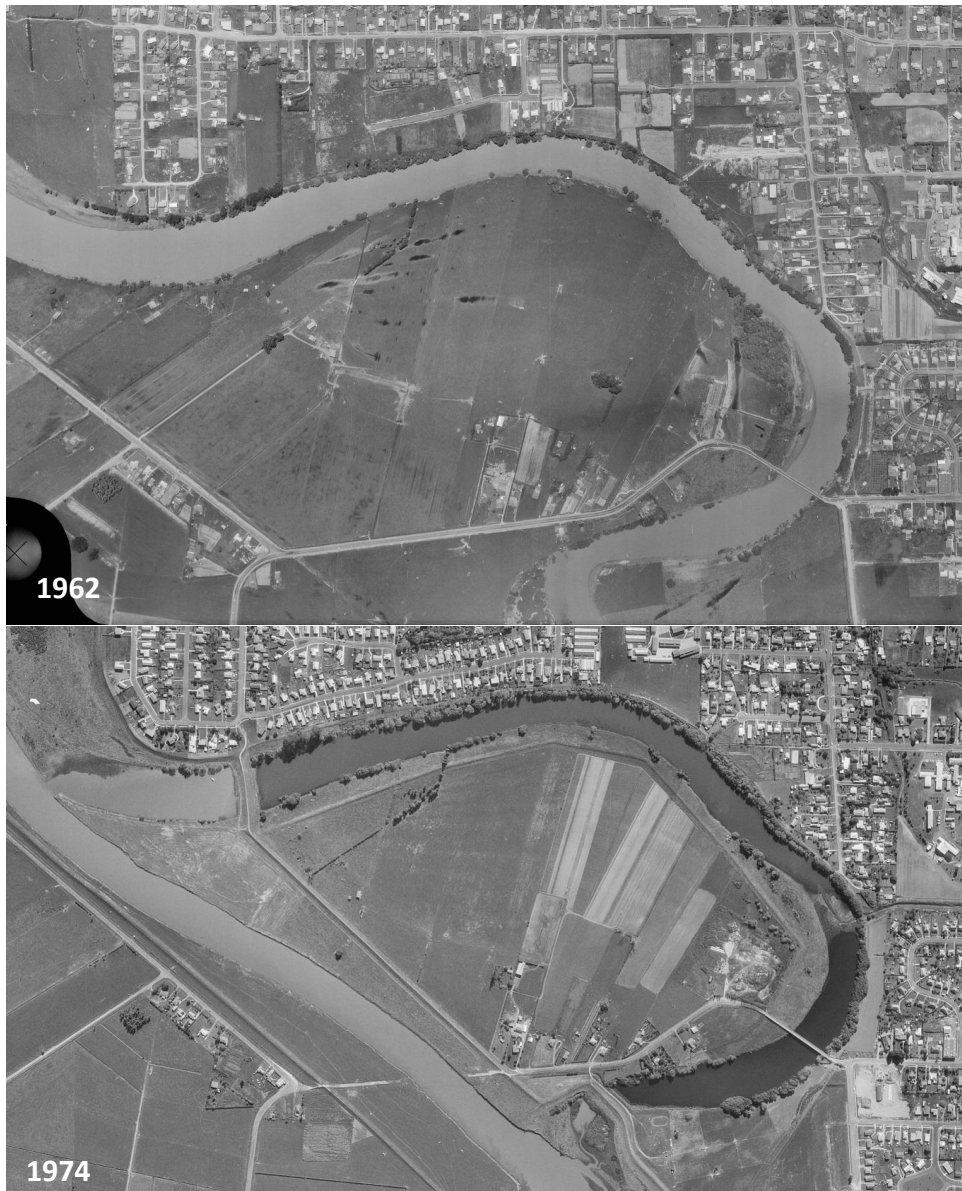
Figure 1.2: Aerial photos of Awatapu Lagoon area in October 1962 before diversion of the Whakatāne River and of the Wainui Te Whara Stream (top); and in April 1974 after the diversions and creation of the Awatapu oxbow (bottom) (Source: Retrolens).
