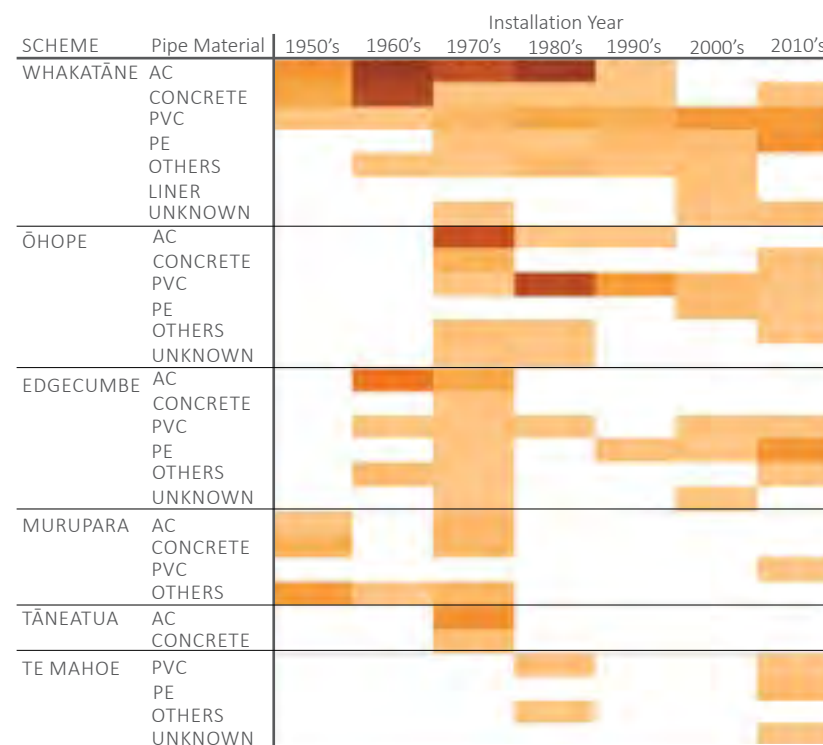
Figure 1: Pipe material and age for each scheme
