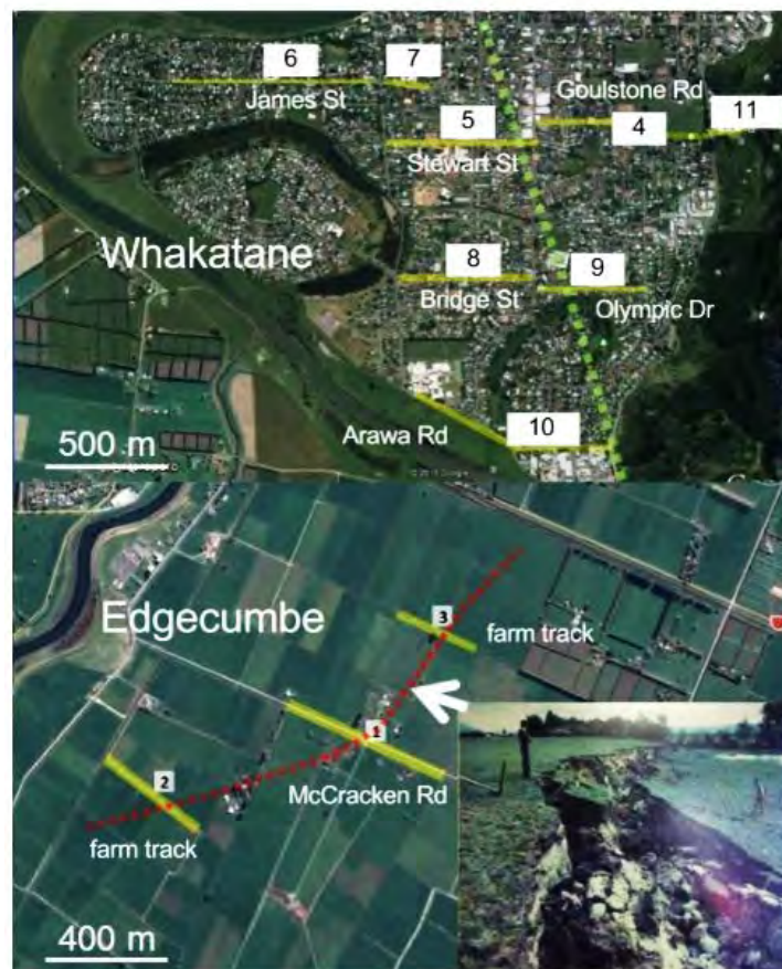
Figure 4.1 Overview of the survey area and seismic profiling map (yellow lines) at Edgcumbe (lower) and Whakatane (upper) survey sites. At Edgcumbe, the red dotted line marks the fault scarp of the 1987 rupture, the green dotted line marks the linear extrapolated Whakatane Fault trace from its known location south of the city. Street names: 1 - McCracken Rd, 2,3 - farm tracks, 4 - Goulstone Rd, 5 - Stewart St, 6,7 - James St, 8 - Bridge St, 9 - Olympic Dr, 10 - Arawa Rd, 11 - Gorge Rd.
