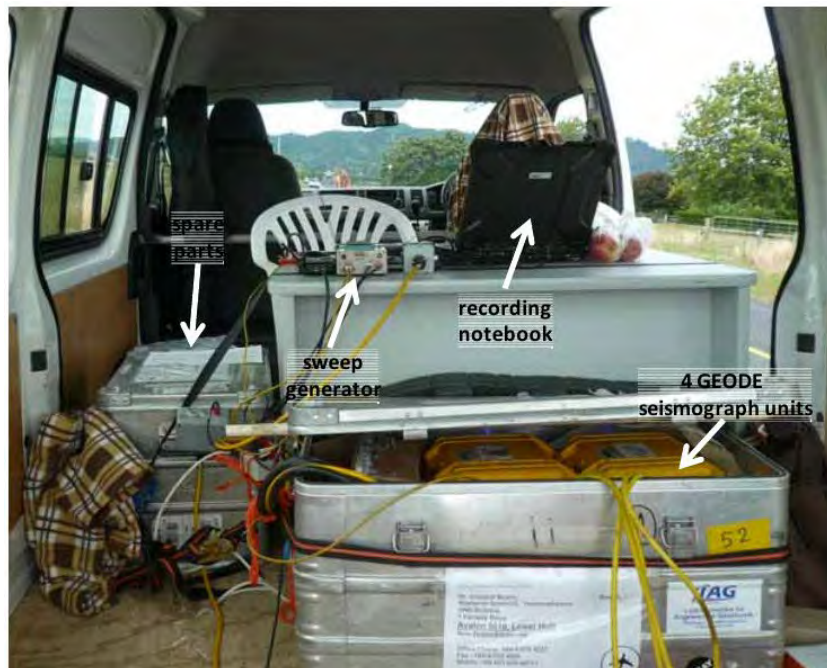
Figure 4.4 Recording equipment installation in the recording car and operators place. The yellow boxes within the aluminium box contain four GEODE seismograph digitizers connected to the recording notebook by an ethernet line. A pack of four 12 V batteries of 160 Ah in total are stored hidden below the table to enable sufficient power supply for several days. The sweep generator on top of the table creates the desired frequency modulated chirp signal (sweep) real time from a digital storage EPROM and initialises precisely the start of the data recording. The signal is sent parallel to the source and the recording system.
