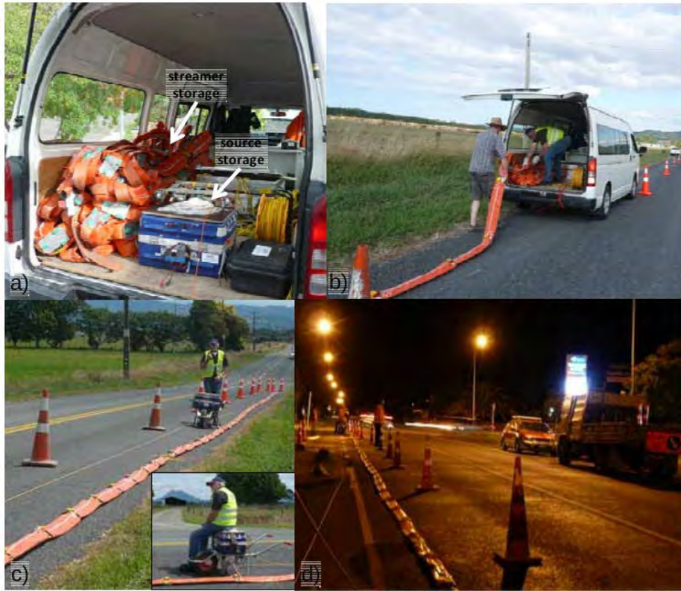
Figure 4.3 Seismic land streamer receiver system (developed by LIAG and GEOSYM): a) during transportation including the dismantled source system; b) during release on site; c) during recording operation on Edgcumbe Fault slope site; d) during night operation in Whakatane. The geophone system was permanently connected to a GEODE seismic recording unit of 96 channels within the recording car at the front of the streamer, from where the recording operation was managed.
